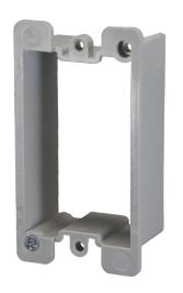
EZSO-EXT EZ BOX PVC Old Work, 1-gang Box Extender is great for remodeling (old work) projects where boxes are set too deep in the wall and need extending. It can extend switch & outlet boxes up to 1-1/8 inches. It can be used with most standard 1-gang nonmetallic electrical switch and outlet boxes.
